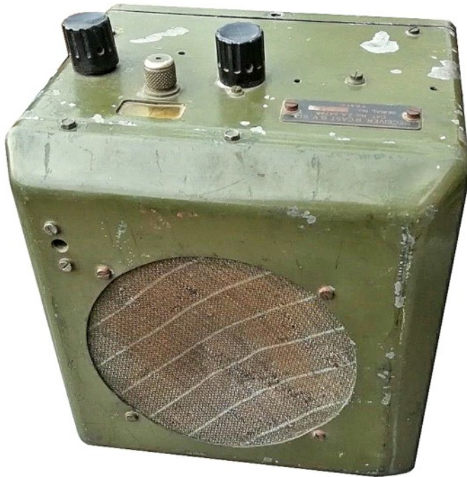
General view of a BV-613 receiver which was principally similar in appearance to the BV-611 and BV-612. A carrying handle on the top panel was not fitted on the BV-613.
