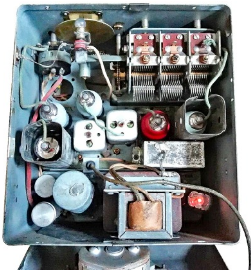
Top view of BV-613 chassis with loudspeaker cover detached.
